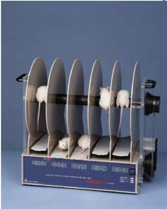
The rat is placed on a horizontally oriented, rotating cylinder (rod) suspended above a cage floor, (not high enough to injure the animal, but high enough to induce avoidance of fall).
